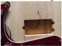
Feed the pickup wires into the control cavity, connect and solder the wires as per the wiring diagram the last page.
