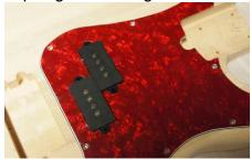
The pickups are mounted with the springs on the screws under the pickups. Only tighten half the way. These screws are for the pickup height adjustment.
